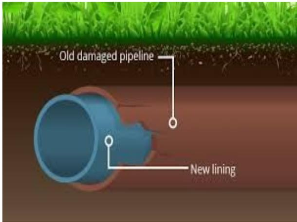
**Hix Plumbing Services** offers an Environmentally friendly, non - invasive trenchless "Pipe Rehabilitation Service" which, in effect, installs a new pipe inside the old existing pipe using a time hardened resin epoxy liner. This process is also known in the standards as CIPP "Cured-In-Place-Pipe"
